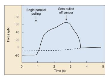
The sliding step experiment. The adhesive force of a single seta was measured. An initial push perpendicularly put the seta in contact with the sensor. Then, with parallel pulling, the force continued to increase over time to a value of 60 microNewtons (after this, the seta began to slide and pulled off the sensor). In a large number of similar experiments, adhesion forces typically approach 200 microNewtons.
