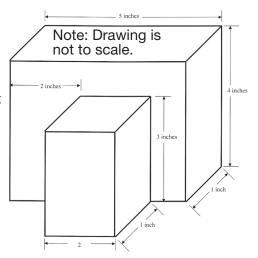
**2. Starting Hint** Determine which views of the object are the most critical to its design. These views should be selected for the orthographic sketch. Often, engineers will use the top, front, and side (right or left) views.
